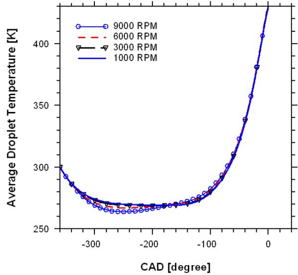
Fig. 5 Average droplet temperature value versus crank angle degree (CAD) for different engine speeds.
