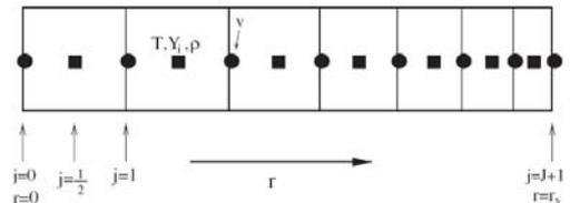
Fig. 1 Schematic of one-dimensional grids for the interior of single droplet simulation adopted from [5].
