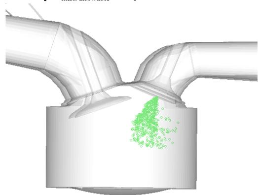
Fig. 7 A typical GDI spray pattern predicted by KIVA-3V for a proposed GDI motorcycle engine.
