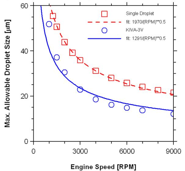
Fig. 6 The maximum allowable droplet sizes for different motorcycle operational conditions. Both predictions can be scaled well by  $D_{\text{max. allowable}} \sim 1/\sqrt{RPM}$ .
