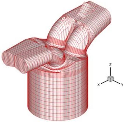
Fig. 2 Grid system used in KIVA3-V R2 simulation.
