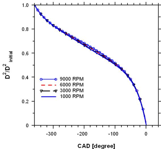
Fig. 4 Square of droplet diameters normalized by their initial values versus crank angle degree (CAD) for different engine speeds.
