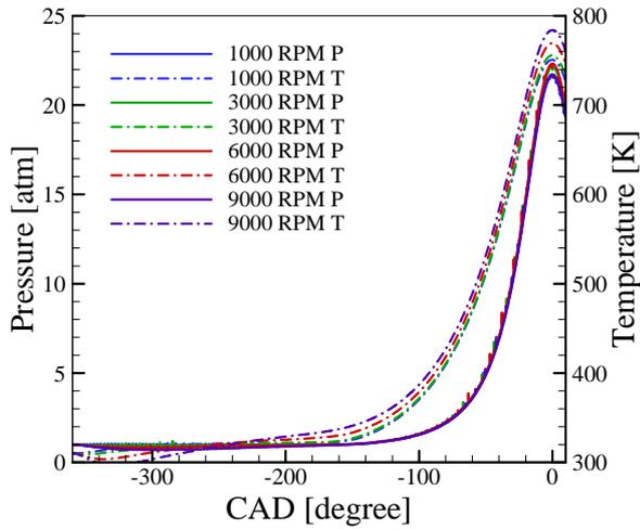
Fig. 3 Pressure and temperature time histories inside the GDI engine motoring for different engine RPMs.
